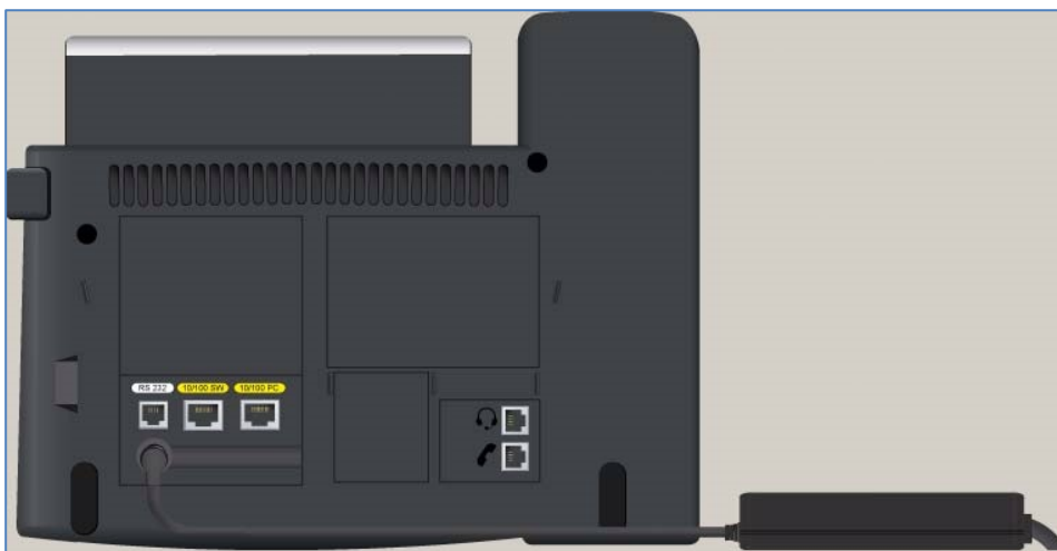
Figure 5.5 Appearance of the bottom part of the IP phone after connecting the power supply
